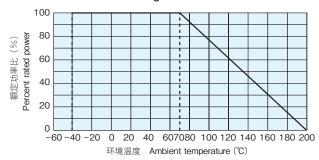
在环境温度 $70^{\circ}$ 以上使用时,7 应按照左图负荷特性曲线,减小额定功率。 For resistors operated at an ambient temperature of  $70^{\circ}$ C or above, a power rating a shall be derated in accordance with the derating curve on the left.
